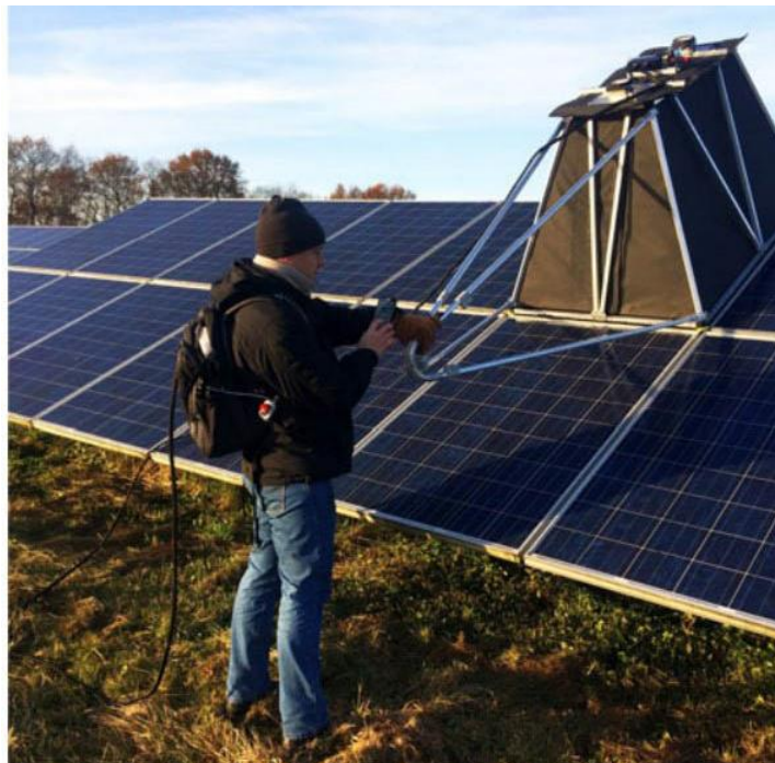
Figure 4: Hood-structure for UVF Imaging in the field at daylight, (2017) [6] p.2
