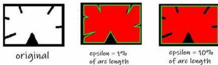
Figure 31: The influence of the tolerance epsilon at contour approximation, [18]
