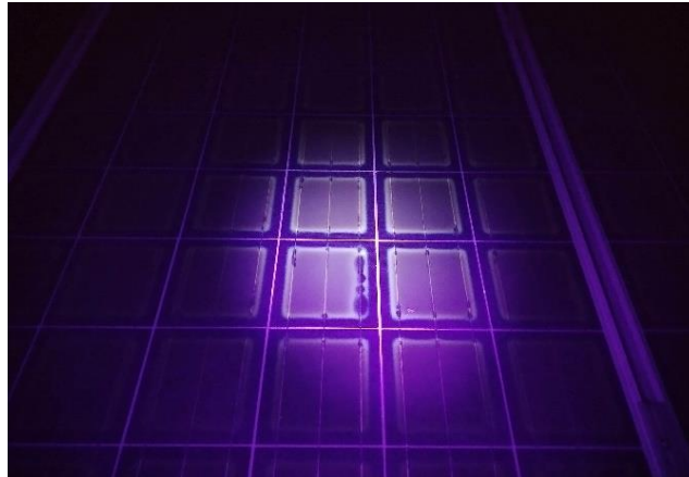
Figure 20: UVF image acquired on 25/04/2022 at Tubarão with the first setup, about 4 cells are well-illuminated
