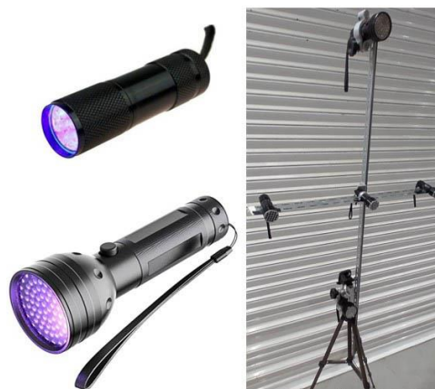
Figure 21: Second setup composed of three 18 UV-LED flashlights and two 51 UV-LED flashlights
